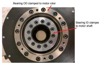
Fig. 1: Bearing assembly schematic
